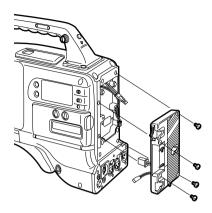
**2** Connect the unit's connectors with the connectors of the AU-M402H battery case.
